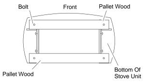
Figure 8 - Removing Pallet Wood From The Bottom of The Stove
